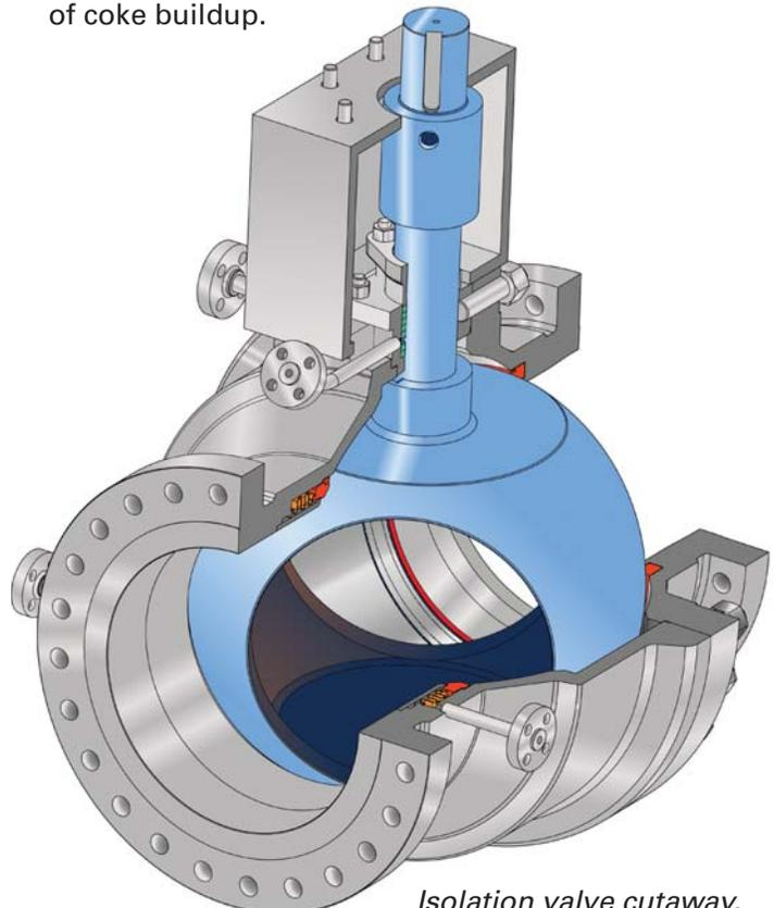
*Isolation valve cutaway.*
